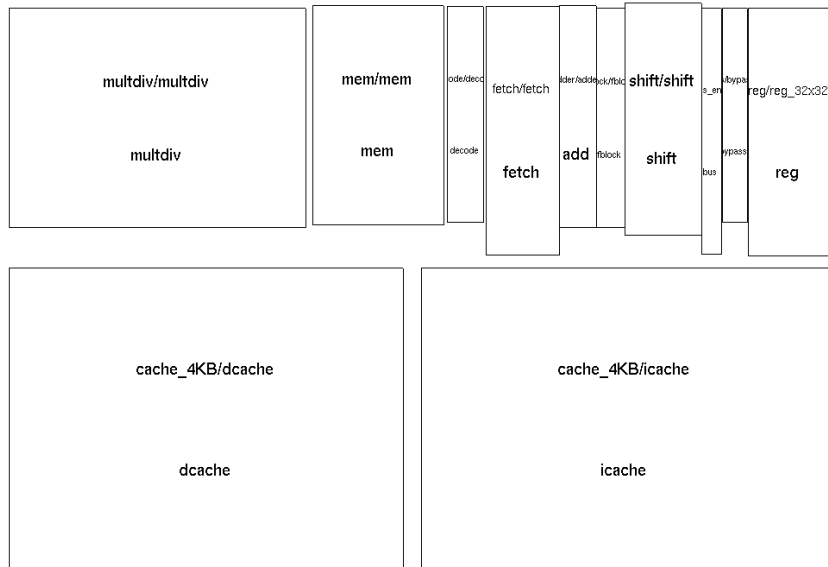
Figure 4. The floorplan for the MiniMIPS
