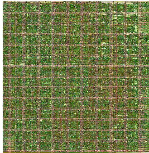
Fig. 4: Routed example design in a 65nm process. Detailed routing was performed using a commercial EDA tool.
