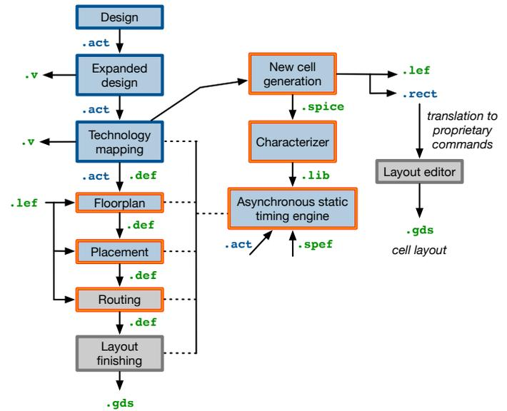
Fig. 3: Design flow for asynchronous logic.
