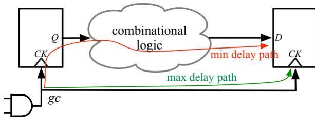
Fig. 1: Hold-time point-of-divergence constraint for generated clock  $gc$ .
