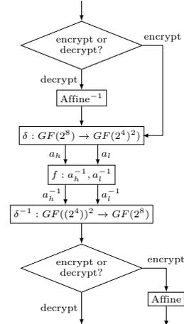
Fig. 5: Composite Field Transformation Byte Substitution
